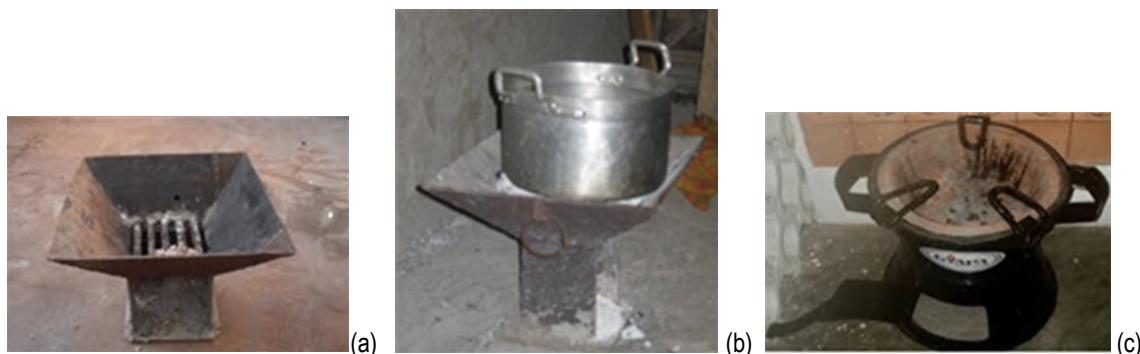
Figure 14: Common Traditional “Coal-Pot” Charcoal Stoves utilized in Liberian households - (a) & (b), and the improved Gyapa charcoal cook stove (c)
