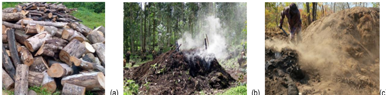
Figure 16: “Mud-Pit” Charcoal production method in common use in Liberia
