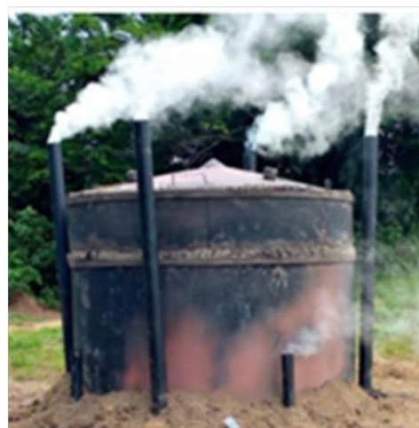
Figure 17: Metal Kiln charcoal production by the National Charcoal Union of Liberia (NCUL) lead by Mr. Richard T.A. Dorbor
